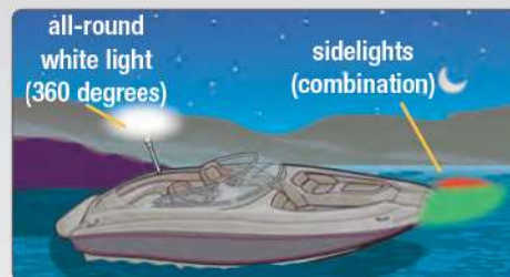
Navigation lights of a power-driven vessel with an all-round white light and combination sidelights placed on the bow
